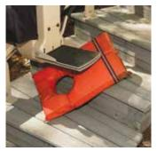
Footrest/carriage safety sensors stop the unit when obstruction encountered.
